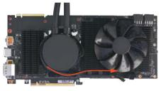
9. Position the shroud adjacent to the graphics card by using the tubes as a reference. Carefully connect the RGB LED connector on the shroud to the RGB header, circled in the image below. Take care that the cables remain away from the fan.
