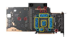
Align the backplate mounting holes and lower the backplate onto the PCB.
