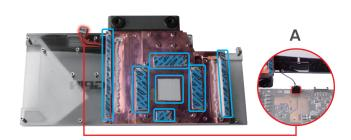
14. Gently lift and rotate the graphics card so that the GPU faces the waterblock. Carefully line up the mounting holes and lower the card onto the waterblock.
