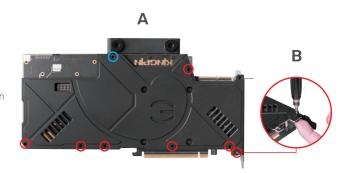
16. Connect the OLED connector to the OLED header on the graphics card (Figure A.), then fasten the OLED to the card (Figure B.) with 4 OLED screws (circled in red).
