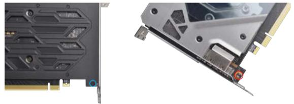
At this point, your waterblock should be fully tightened and ready to test. As noted before, please use care to avoid overtightening, as this may strip the screws and/or damage the graphics card. Lastly, do not use power tools to install the waterblock or backplate.
