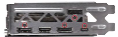
(b) For #C and #E models, remove the screws circled on the bracket to the right with a Phillips #1 screwdriver and set the screws aside, You will need to put it back after installation of waterblock.
