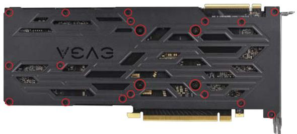
2. (a) For #A, #B, and #D 2slot models, remove the screws circled on the bracket below with a Phillips #1 screwdriver and set the screws aside. You will need to put it back after installation of waterblock.
