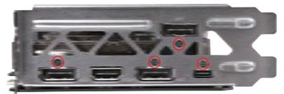
(b) For #C and #E models, remove the screws circled on the bracket to the right with a Phillips #1 screwdriver and set the screws aside, You will need to put it back after installation of waterblock.
