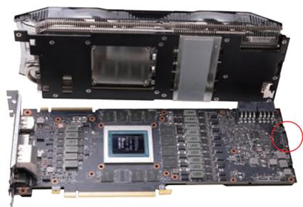
(b) Please be careful when removing the fan and LED connector, the wires can snap if pulled too hard. The safest way to remove the connector is with a small flat-head screwdriver, tweezers, or fingernails to raise the edge of the headers a little at a time. Set aside the heatsink/fan; it will no longer be needed for this Kit.
