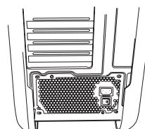
3. Use the screws provided with your case to install the power supply into your computer. **NOTE:** It is recommended to install the power supply with the fan facing down. However, if your case places the power supply at the bottom of the case and there are no ventilation holes available, it may be best to install the power supply with the fan facing up for greater efficiency and reliability.
