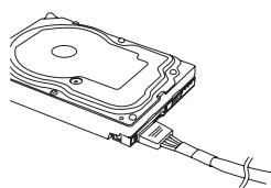
8. Connect the peripheral “Molex” 4-Pin connectors for fans, pumps, legacy components and other devices/adapters.
