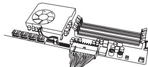
5. Connect the 4+4-Pin EPS12V cable to the motherboard.
