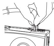
7. Connect SATA power cables to all data drives or optical drives (hard drives, solid state drives, optical drives).
