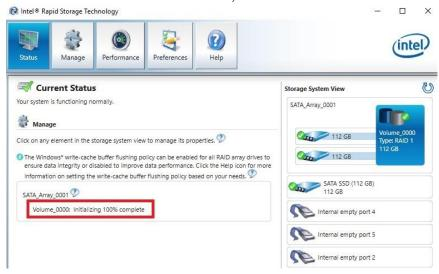
If you select the "Manage" tab, you can see a bit more in-depth information on the array and additional options to manage or change the array.
