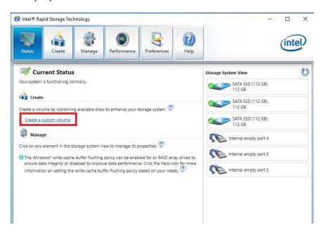
This guide will illustrate how to create a RAID1 array using the IRST. Using the screen above, we know that three (3) SSDs are currently attached to the controller and the other three (3) INTEL® SATA ports are empty (this can vary board to board based on how many Intel® SATA ports are present). If you plan to create another type of array, please ensure that you have the correct number of drives attached and shown on the status screen in IRST for your intended array before you start.
