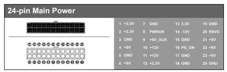
**ATX\_PWR\_24p** is the main power supply connector located along the lower-right edge of the board. Make sure that the power supply cable and pins are properly aligned with the connector on the motherboard. Firmly plug the power supply cable into the connector and make sure it is secure.
