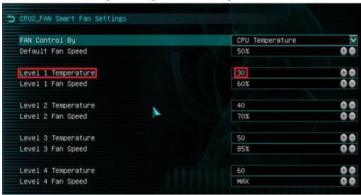
There are four tiers of temp control, with Level 4 fan speeds generally recommended to be set at Max. The example above uses a fairly aggressive fan curve, but you can set this as high or low as you wish. Make sure, however, to stay below 5-10C of the Max safe load temp for your specific processor, which can be found at Ark.Intel.com. All Smart Fan Settings have the same controls and can be setup the same way.
