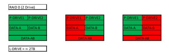
As RAID0 has no fault tolerance, even a single drive failure compromises the array and renders the array Failed and unrecoverable.
