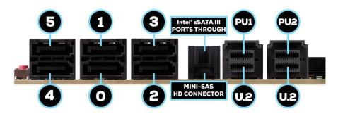
SATA ports on this platform natively support full AHCI and RAID functions. AHCI is enabled by default, but the controller can be put into RAID mode in the BIOS. RAID mode supports RAID levels 0, 1, 5, and 10 through the Intel® controller. RAID-ready ports also have full AHCI functionality.
