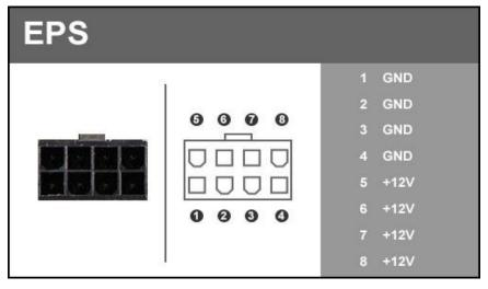
**EPS PWR 8P**, the 8-pin ATX 12V power connection(s), is used to provide power to the CPU. Align the pins to the connector and press firmly until seated. Additional EPS, if present, is optional for improved overclocking. Please remember to make sure that the tab on the EPS socket is aligned with the release clip on the cable.
