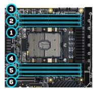
and Cascade Lake-SP. It is recommended to always use a 6 DIMM Hexa-Channel kit for the SR-3 DARK. Fill the memory slots in the following order: 3, 6, 2, 5, 1, and 4. See chart below:
