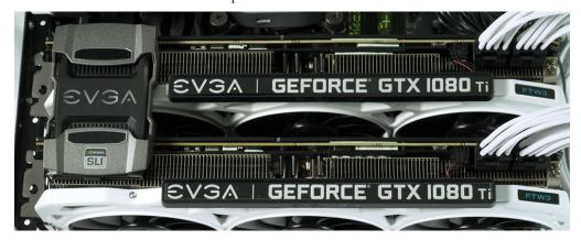
2. After the cards are installed, have power connected, and the SLI/NVLink bridge is attached, boot into Windows. The graphics driver will normally identify the cards and automatically configure the driver. If not, then you may need to reinstall the driver.
