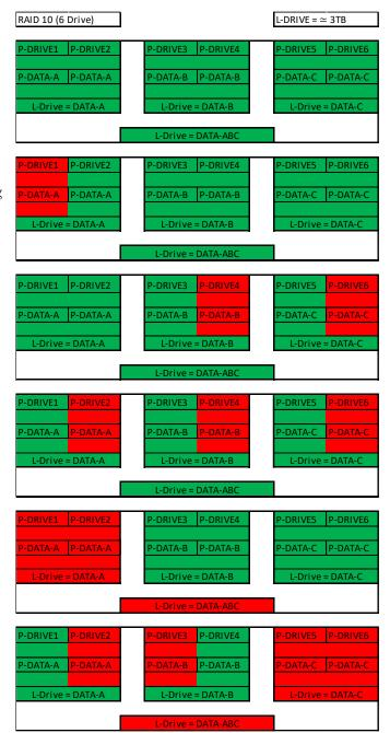
**RAID0+1**: RAID0+1 is a form of nested RAID that was widely used on previous generation boards. <u>Although EVGA C622 series motherboards do not use this type of array</u>, it is listed here to show the improvements made by RAID10, and to clear up a common misperception that RAID0+1 and RAID10 are the same.
