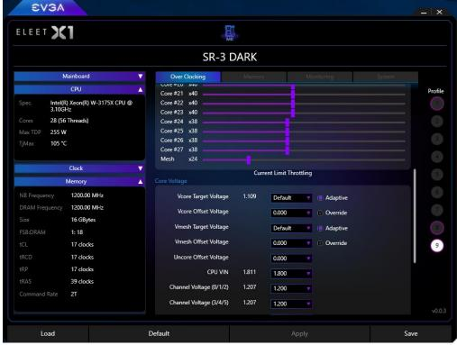
As seen above, there are options for multiple voltages, and two options for your CPU Vcore and Vmesh: Adaptive and Override voltages. Adaptive allows for a tighter voltage profile to keep voltage and heat to a minimum, while Override is more of a brute-force method of setting your voltage. One primary advantage of using a stable Adaptive voltage is that it allows your CPU to properly take advantage of C-States and energy saving features, which can extend the lifespan of your CPU.
