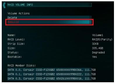
Next, you will see a list of all attached HDD/SSDs that can be used to rebuild the array. Select the disk, then click on it or press enter.
