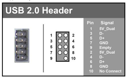
The SR-3 DARK also features an onboard USB 2.0 port header, near the CPU Fan headers. This header has a specific purpose – to allow you to flash the BIOS without an installed CPU using the included USB flash drive. For more information on flashing the BIOS without a CPU, please see Page 143.
