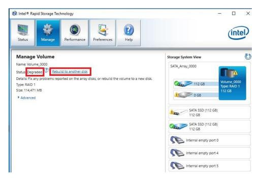
Next to "Status: Degraded," left-click the hyperlink labeled "Rebuild to another disk." This will bring a pop-up window over the IRST showing a list of attached drives that can be used for the repair (see pic on next page):
