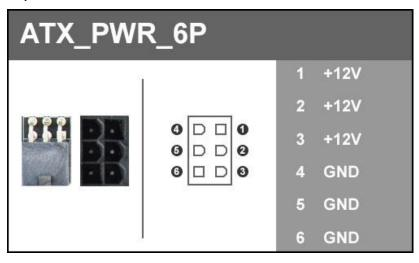
The 6-pin PCIe connector present on the motherboard provides additional power to the PCIe slots, rather than pulling it all from the 24-pin main power. It is advised to plug in this connector when using SLI, especially with higher-end graphic cards. It is strongly recommended to plug in this connector for 3-way and 4-way SLI, regardless of GPU.
