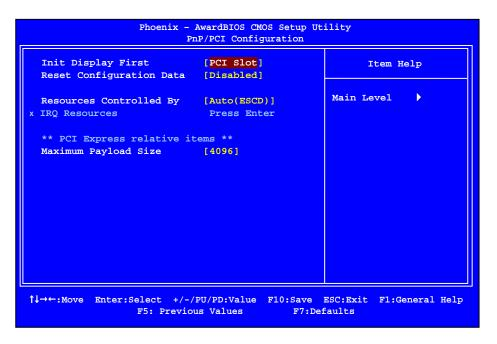
Figure 15. PnP/PCI Configuration Menu
