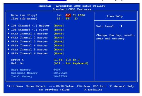
Figure 6. Standard CMOS Features Menu
