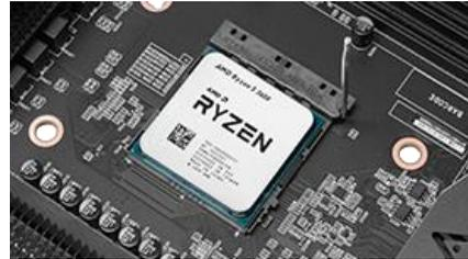
5. Carefully lock the lever back into place by lowering it down to the PCB, and then push the lever towards the socket and down under the hook.
