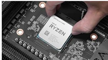
**Note:** The gold triangle key on the CPU should match the triangle key on the socket.
