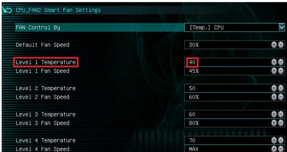
There are four tiers of temp control, with Level 4 fan speeds generally recommended to be set at Max. The example above uses a fairly aggressive fan curve, but you can set this as high or low as you wish. Make sure, however, to stay below 5-10C of the Max safe load temp for your specific processor, which can be found at <https://www.amd.com>. All Smart Fan Settings have the same controls and can be setup the same way.
