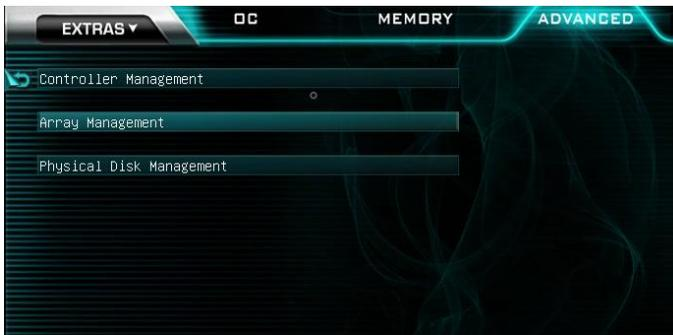
Before you begin, enter the Array Management menu to check if any old arrays are still detected on the physical drives you plan to use. You must delete old, **unneded** arrays prior to creating a new array or using drives previously used in the old array.
