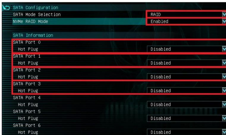
Once RAID is enabled and all devices are detected, press F10 to save and exit. Upon reboot, repeatedly press “Delete” to reenter the BIOS. Once in the BIOS, go back to the “Advanced” tab where you’ll find a new item at the bottom of the list called “RAIDXpert2 Configuration Utility.”
