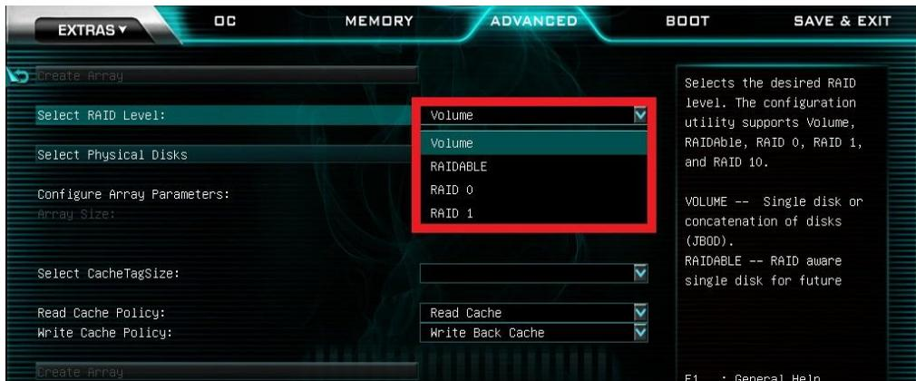
We’ve discussed RAID0, RAID1, and RAID10 in detail above. Volume simply means that you may combine several drives into a single volume, often called a JBOD (Just a Bunch of Disks). RAIDABLE is a more advanced option, which allows you to set aside one or more drives to be configured as an “as needed” drive to create a RAID0 or RAID1; a RAIDABLE drive will not be used unless it is added to or replaces another drive in an existing array.
