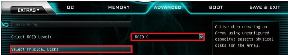
On the Select Physical Disks page, you can sort visible drives via HDD-type drives or SSD-drives (or both), to ensure that you don't mix and match drives in your array. When ready, switch each drive that you intend to add to your array to "On". Once all drives for your array are selected, click "Apply Changes".
