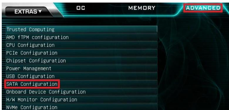
2. Change the SATA Mode Selection to “RAID”, which will add new options for M.2 Key-M PCIe Storage RAID. Set the “NVMe RAID Mode” to “Enabled”.
