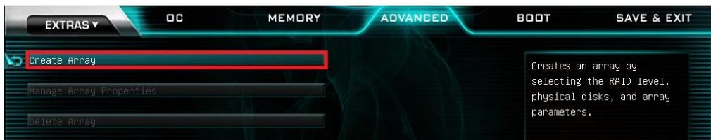
EVGA X570 motherboards support RAID0, RAID1, RAID10, JBOD, and creating a hot spare for an existing RAID (such as RAID1 and RAID10). Click on the dropdown menu for Select RAID Level to see your options:
