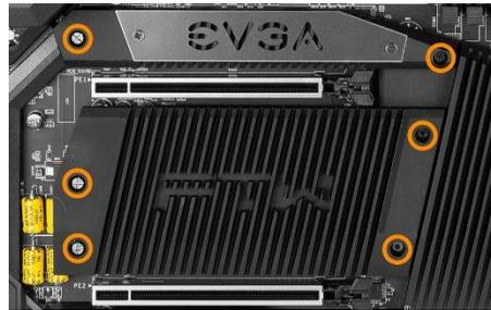
Before you can install a 110mm M.2 device, you must first remove the screw that comes pre-attached to the Socket 3's retention standoff; this will be used to keep the M.2 device in place and also used to secure the heatsinks back in place.
