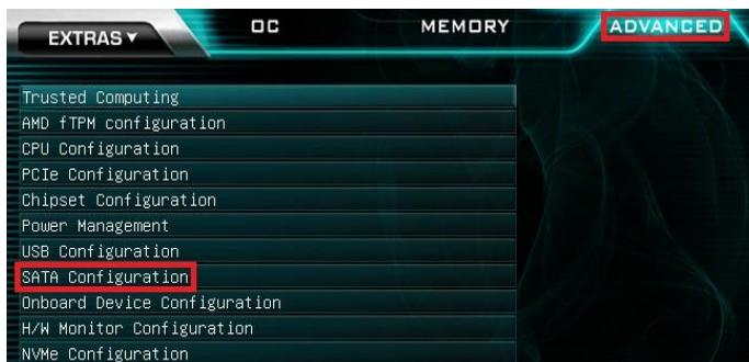
In the “SATA Mode Selection” at the top, the default will be AHCI. Click on the arrow to the right side of AHCI or navigate to it with your keyboard and press “Enter” to open the pulldown menu. Select RAID from the list.
