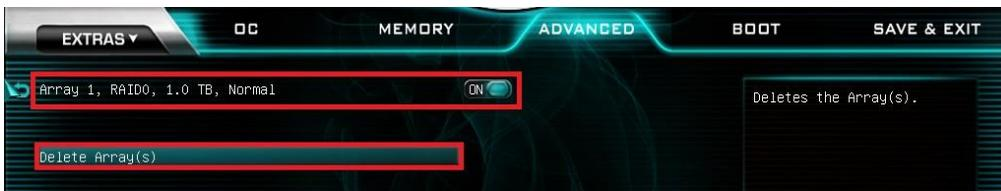
The RAIDXpert2 Configuration Utility will require you to both confirm that you wish to delete the array and ultimately click “Yes” to delete the array.
