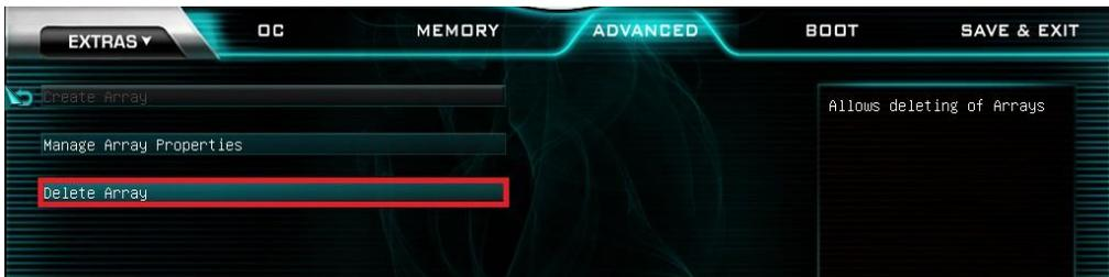
If any arrays are detected, they will be listed on this page. You may select one or multiple arrays to delete on this page by toggling them “On”. It is **strongly recommended** that you make absolutely certain that you are ready to delete the arrays, and that you have removed any data you wish to keep. Once you have selected your arrays to delete, click the Delete Array(s) button.
