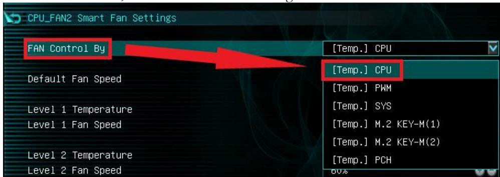
First, choose the temperature monitor the PWM controller will use to monitor for its temp information. It's recommended to link the fan control to the CPU, which is predominantly the most important temperature in the system. The exception is when you have 64GB of heavily overclocked RAM, which may cause PWM temps to be a concern. If this is a concern, set the fan control to the PWM temp.
