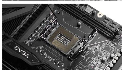
3. Align the notches on the CPU to the notches in the socket, and lower the processor straight down into the socket.
