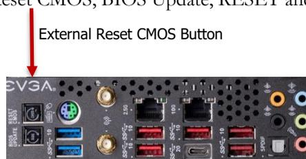
Use the Reset CMOS button to clear the BIOS before and after updating the BIOS, and as a troubleshooting option when the motherboard fails to POST (e.g. after installing new hardware, testing an unstable overclock, etc.).
