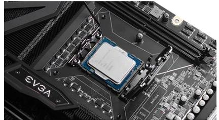
4. Lower the load plate so that it is resting on the CPU, and make sure to slide it under the lever's loop.
