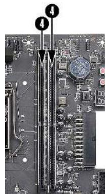
Use the following procedure to install memory DIMMs. Note that there is a key notch near the center of the DIMM slots. This matches the gap on a DDR4 DIMM to ensure the memory is installed properly, and to prevent the incorrect installation of memory.
