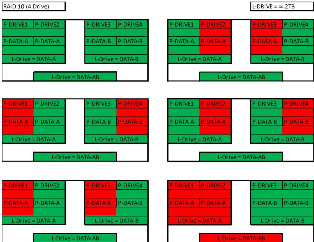
While the Z370 MICRO controller will support a four or six drive RAID10 array, RAID10 can scale indefinitely provided the controller supports more drives. Every pair of drives adds an additional mirrored node, which increases the theoretical number of failures the array can suffer before a loss of data occurs. However, an array can still fail due to both drives on a node failing.
