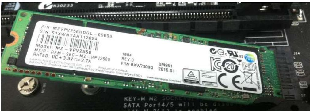
3. Gently push the M.2 device down on the raised end. There will be some tension - this is normal - then use the screw you removed in Step 1 to secure the device. Below, you can see that the contacts will be nearly invisible when the device is properly seated and the copper mounting semi-circle is partially visible around the screw.
