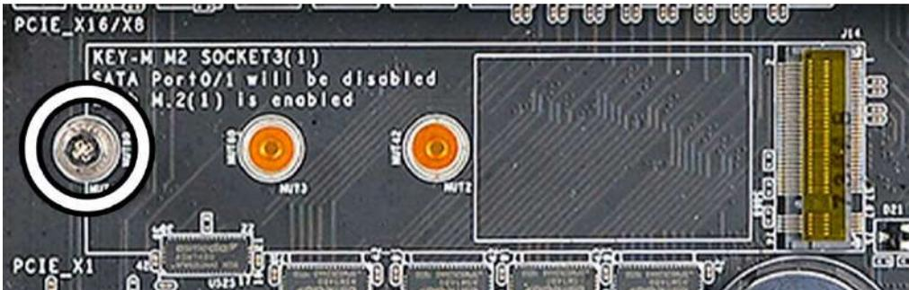
2. Insert the M.2 device at a slight angle - approximately 45 degrees to the board. This will allow the contacts (colloquially called “Gold Fingers”) to seat completely into the slot. If the device is fully seated, you should be able to release it and the device will rest at an angle of about 30 degrees on its own, as shown in the picture below.
