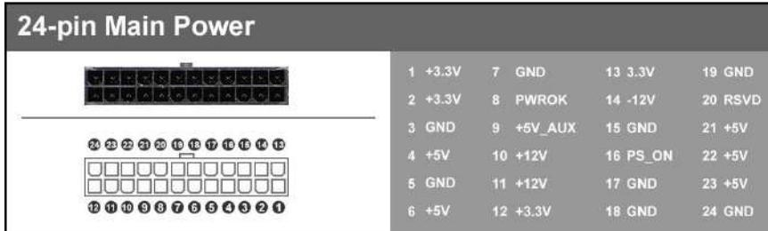
ATX\_PWR\_24p is the main power supply connector located along the lower-right edge of the board. Make sure that the power supply cable and pins are properly aligned with the connector on the motherboard. Firmly plug the power supply cable into the connector and make sure it is secure.
