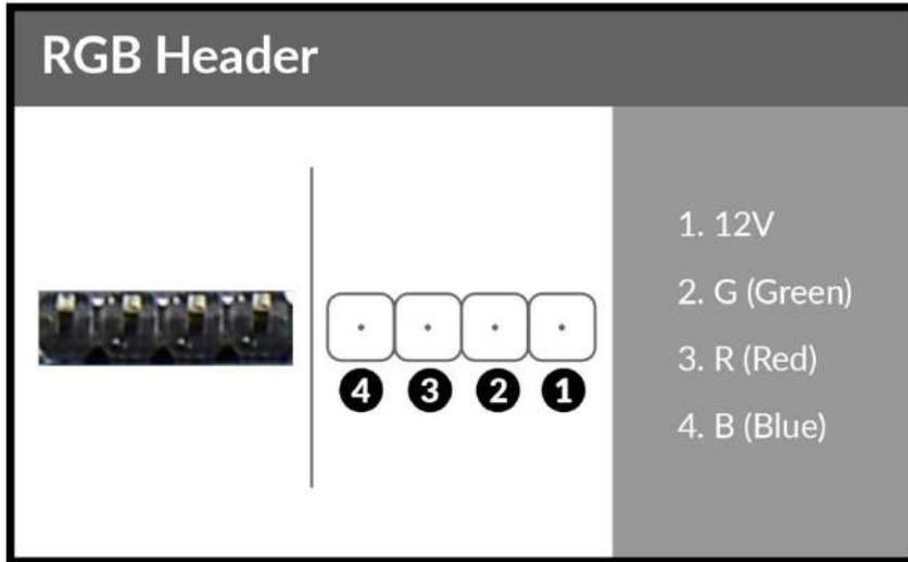
This header and pinout is also shared with the RGB LED header, which also supports 1 Amp @ 12 Volts (12 Watts). This will add control options through EleetX for controlling RGB LED's.
