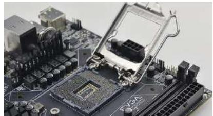
3. Align the notches on the CPU to the notches in the socket, and lower the processor straight down into the socket.
