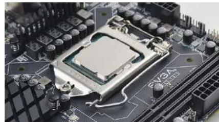
**Note:** After removing the CPU socket cover, it is recommended to store it in case you ever need to transport your motherboard. If you ever remove the CPU, it is highly recommended to reinstall the socket cover.
