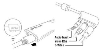
1.Connect the AV-input adapter (included) into the input located on the rear of inDtube next to the gold platted MCX input. The AV-input on inDtube is notched and will only fit one way. Do not force in as this may cause irreversible damage to both the AV-input adapter and inDtube.
